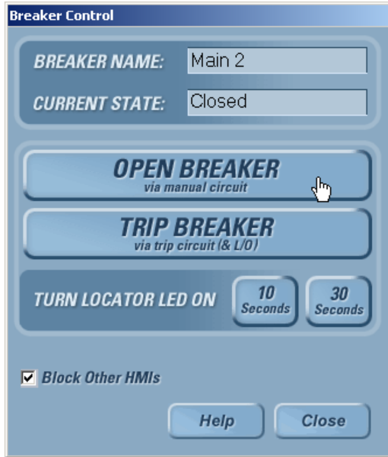
Figure 4-6 Breaker Control screen
